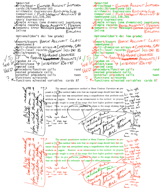
Figure 8. Handwritten annotation and machine print discrimination captures annotations although some annotations cause false positives.
