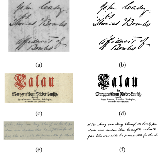
Figure 2. Samples of the test dataset resulted from binarization using localization of object-of-interest 2(b): image binarization of 2(a), 2(d): image binarization of 2(c), 2(f): image binarization of 2(e)
