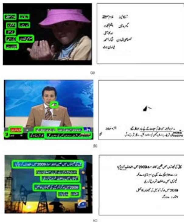
Figure 4. Text localization and extraction results for video images taken from different sources. (a) Movie credits (b) News tickers (c) Oil prices
