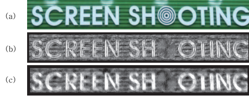
Figure 3. Example of contextual feature. (a) Input image. (b) Text confidence by local features. (c) Text confidence by contextual feature.
