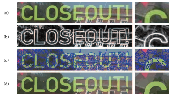
Figure 2. Procedure for constructing superpixels. (a) Input image. (b) Edge map of (a). (c) Superpixel image (boundaries of superpixels are marked as blue lines) (d) Quantized image with average colors of superpixels.
