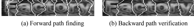
Figure 4. Two-pass path finding algorithm. In (a), different starting points converge to the same end points. In (b), the false cuts going ‘F’ have been removed while the true cuts are retained.
