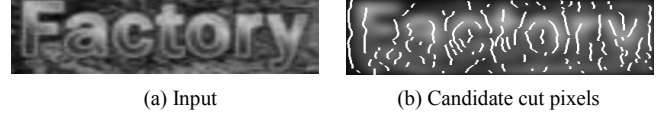
Figure 3. Candidate cut pixels of a sample image. In (b), the image is blurred to make the (white) cut pixels more visible.
