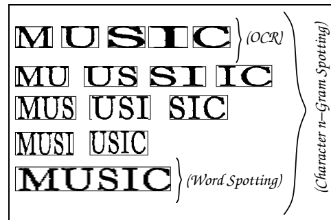
Figure 1. Traditional approaches index/recognize either characters or words. In contrast, our approach indexes the character n-grams, i.e. groups of consecutive characters in the word. With our framework, we fill a major gap in the problem space, while scaling spotting techniques to large vocabulary and document collections.
