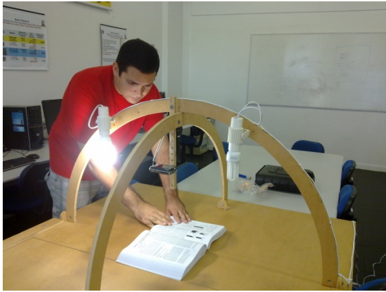
Figure 2 – Digitization platform with two light sources and portable digital camera ( UFPE-Planetarium ).
