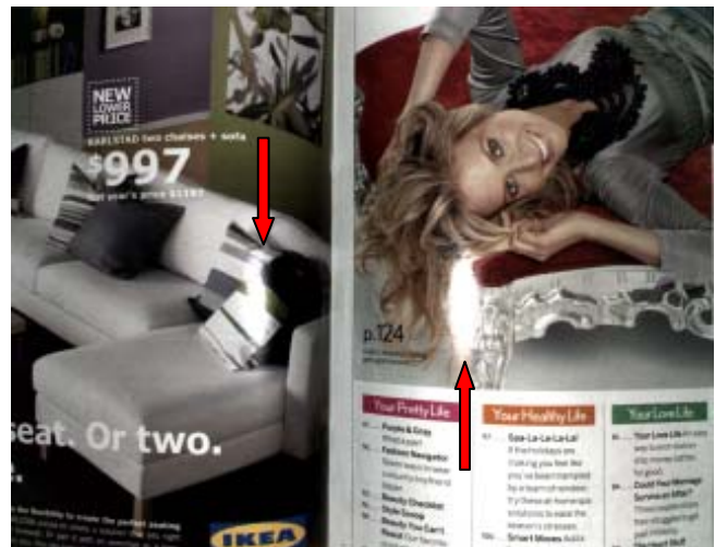
Figure 1. Photo of a two page magazine printed on glossy paper with specular noises.
