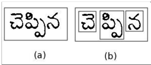
Figure 5. (a) A word image (b) aksharas (shown in rectangles) obtained after character segmentation on the word image shown in (a).
