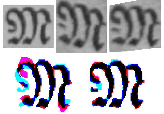
Figure 3. Gothic "M" character distortion correction. Top row (from left to right): "M" super-symbol, original "M" character and "M" after correction; bottom: difference maps before (on the left) and after correction
