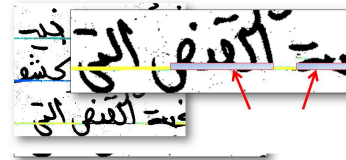
Figure 5. Using the average thickness of a rule-line estimated from its line pattern, the thick areas are marked out (pointed by arrows). The rest of the pixels in the line pattern will be used in the linear regression estimation of a best fitting line.
