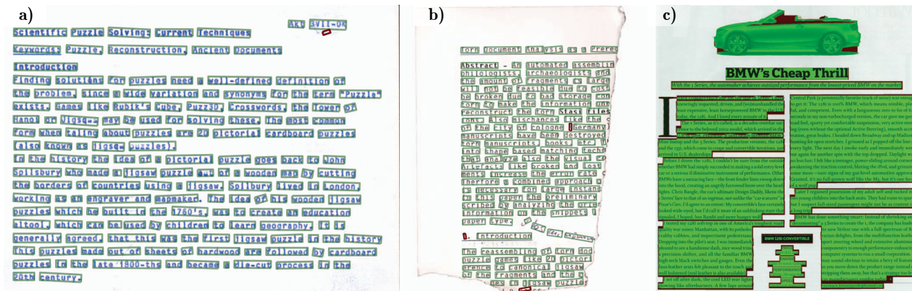
Figure 4. A carbon copy (a), a machine printed snippet with annotations (b) and page from the PRImA database (c). The light (green) rectangles in (a,b) indicate correctly classified text while dark (red) rectangles mark false classification results. In (c), light (green) areas illustrate true positives, while dark (red) areas indicate false positives and false negatives.
