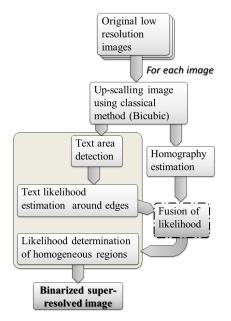
Figure 1. Block diagram of the proposed algorithm. The FAIR algorithm is represented in gray.
