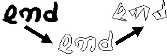
Figure 1: This image illustrates how contours and edges are extracted from connected components in documents.
