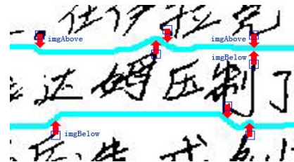
Figure 2. Red arrows represent the effects of the foreground pixels on the paths drawn in cyan. The rectangular regions of imgAbove and imgBelow are marked by blue rectangles.
