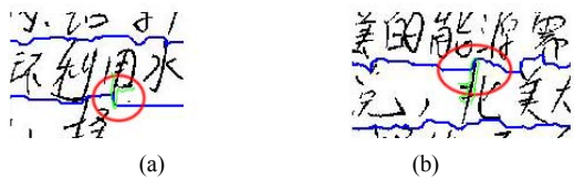
Figure 5. Green curves represent the contour of the CCs. Red ellipses mark the area where the path bypasses the foreground pixels following the contour of the CCs.
