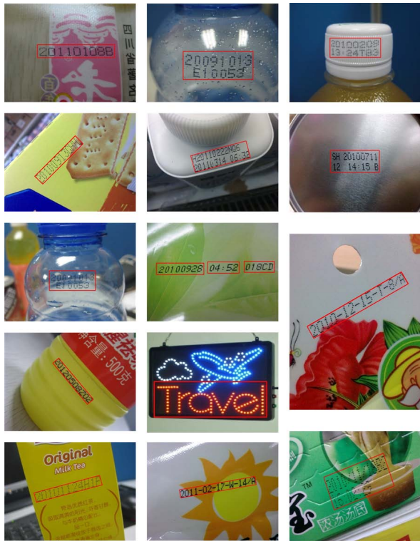
Figure 8. Additional examples of dot text detection. The results are marked with red rectangle.
