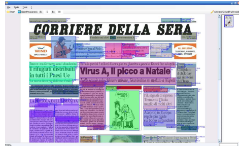
Figure 4. A screenshot of the software tool, in the evaluation phase of an article identification algorithm. Here, blocks with the same color belong to the same article.
