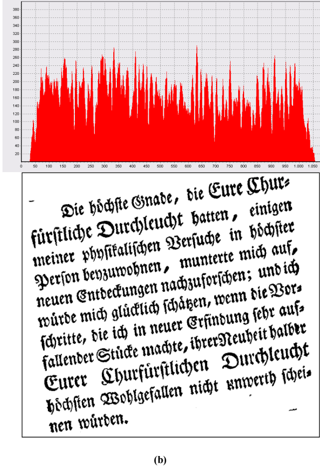
Figure 3. The histograms of a deskewd (a) and a skewed (b) image show the contribution of the black borders of the page when it's aligned.
