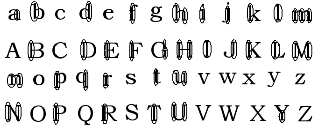
Figure 1. The latin alphabet with the major vertical strokes circled. There are secondary vertical strokes which also contribute in the performance of the proposed method.
