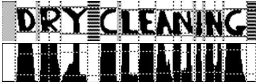
Figure 5. Vertical projection analysis for character segmentation.
