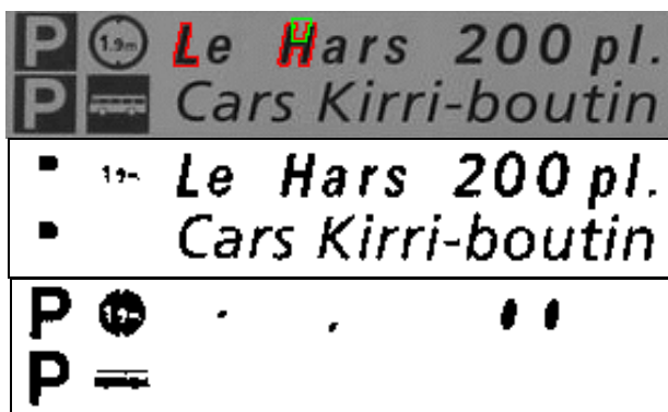
Figure 5. Top - original with close contour of "good" CC (red) and artifact (green) of inner part of "H" character; middle and bottom - non-reverse and reverse video text layers, respectively.
