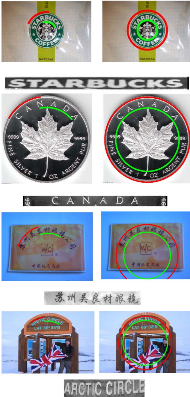
Figure 4. Curve TILT method. The top left image is the input image, the top right image is the result of curve TILT method. The bottom image is the circle ring expansion result.
