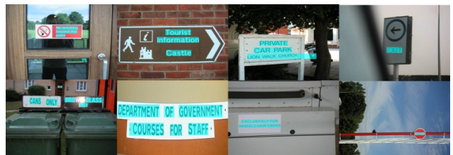
Figure 5. Some example results of text string detection on the Robust Reading Dataset. The detected regions are marked in cyan.
