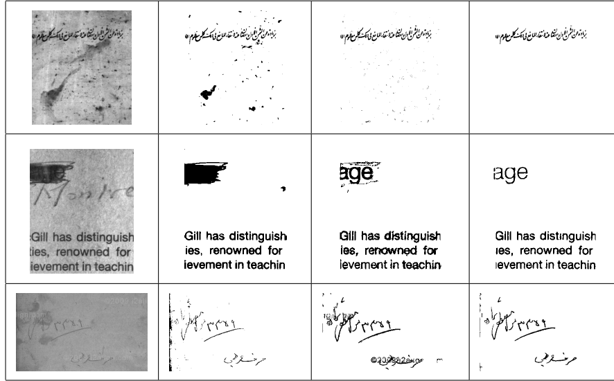
Figure 3. Subjective comparison. From left to right: original images, AdOtsu outputs, ML with only reflectance components, Proposed method outputs.
