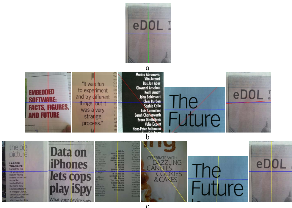
Figure 2. Examples of the catastrophic errors produced by the algorithms. (a) The only catastrophic error produced by the proposed algorithm. (b) Examples of catastrophic errors produced by the Projections method. (c) Examples of the catastrophic errors produced by the Traditional Hough method. Blue lines: ground truth orientation, green line: orientation computed by the proposed method, red line: orientation computed by the Projection method, yellow line: orientation computed by the Traditional Hough method.
