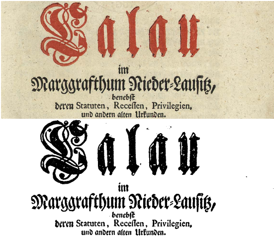
Fig. 1. Binarization of a print document from the DIBCO-09 test set.
